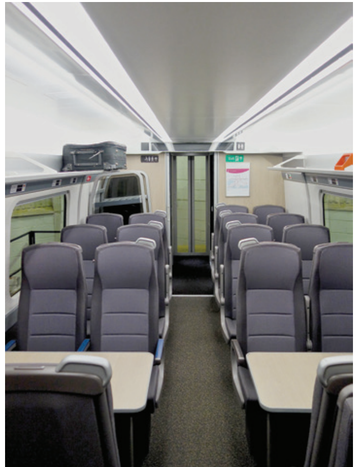
Standard Class saloon with LED lighting and overhead luggage rack.. John Whitehouse
