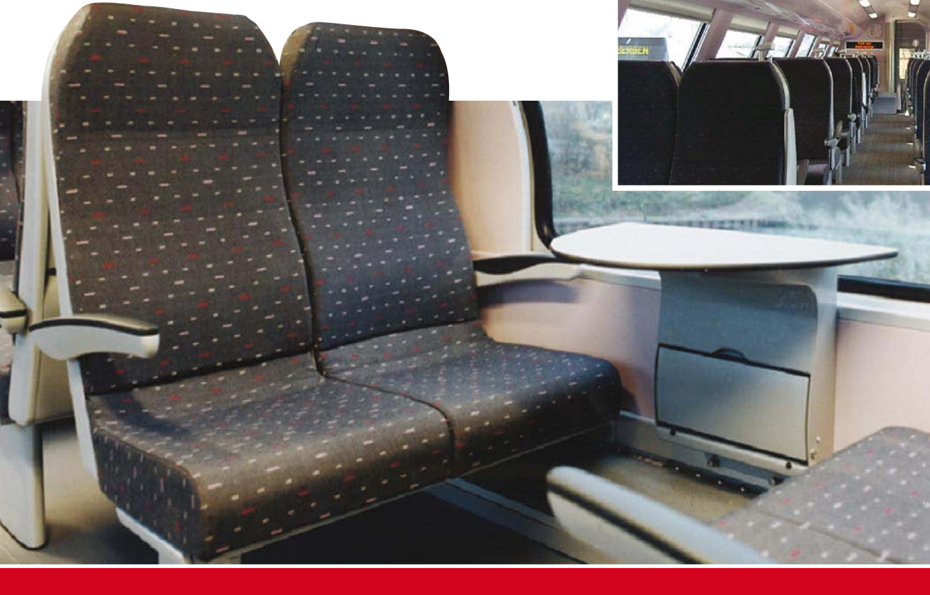
ABOVE: Upper saloon showing staggered seating and window bays LEFT: Typical seating bay
