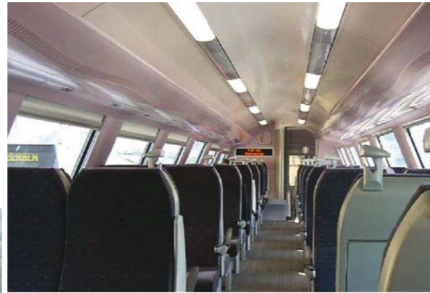
ABOVE: Upper saloon showing staggered seating and window bays LEFT: Typical seating bay
